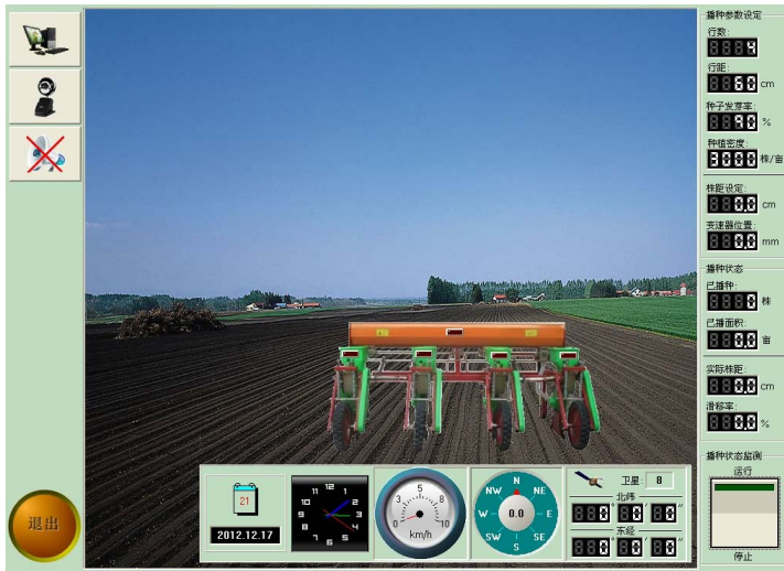
Figure 7 System interface of for planter's working status monitoring working status of planter
